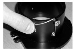
Release the springs on both sides of the adapter (press out from the adapter body).
